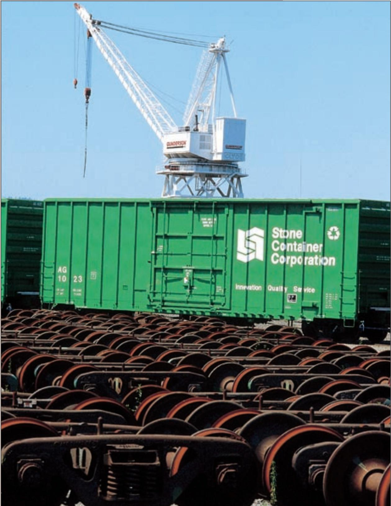
*Truck assemblies stored prior to refurbishment form foreground to new forest products boxcars as they move along Gunderson's delivery track. The 200-ton capacity shipyard crane is in background.*
