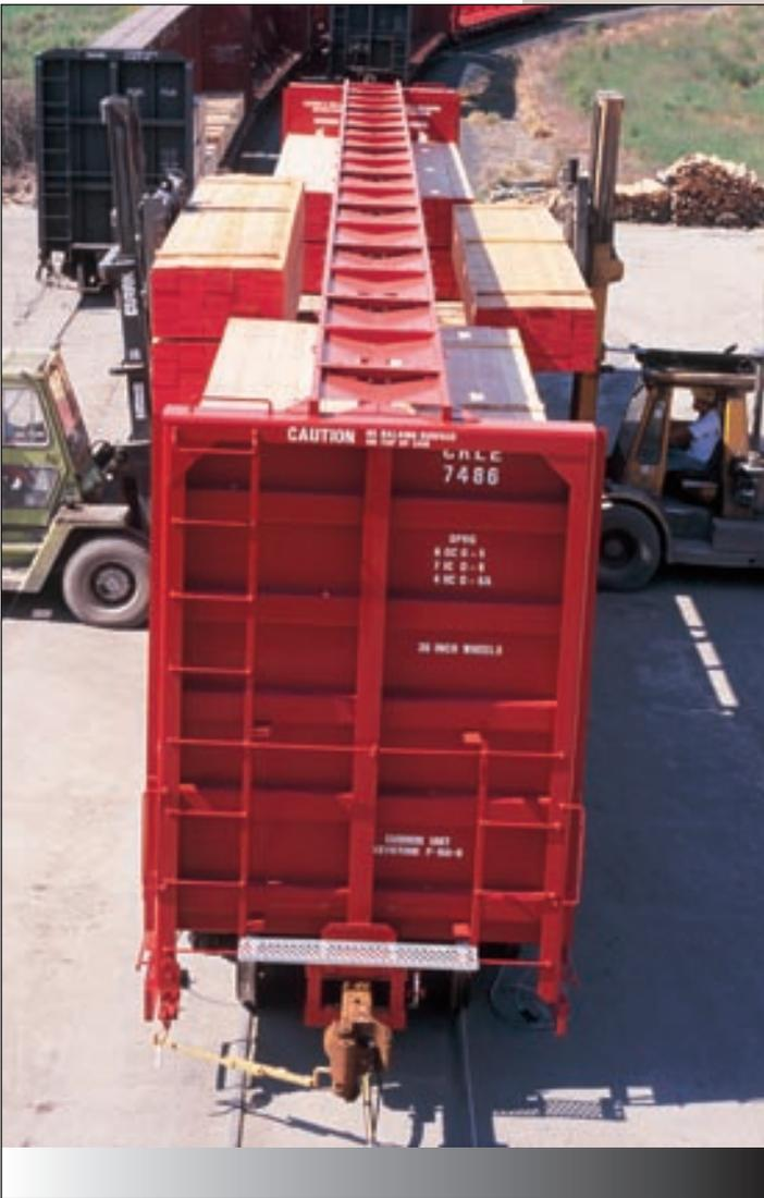
*Above: Center partition cars brought greater capacity and efficiency to hauling lumber by rail. Loading is simply performed from both sides of the car.*
