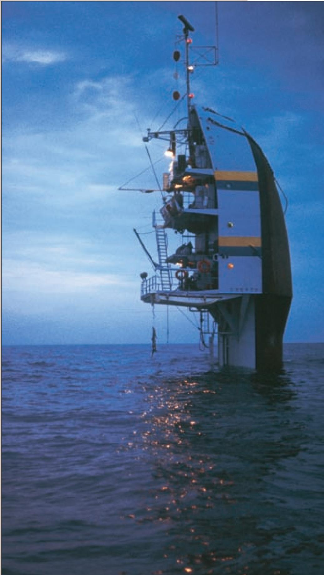
*“Flip,” a floating instrument platform, launched in 1962, shown at work in the Pacific Ocean during research by the Scripps Institute of Oceanography in 1963.*
