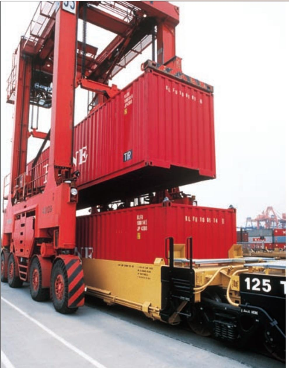
*Maxi-Stack I was the first non-bulkhead car, which had 125-ton trucks at the articulation and much higher weight carrying capacity per forty-foot well than Twin-Stack.*
