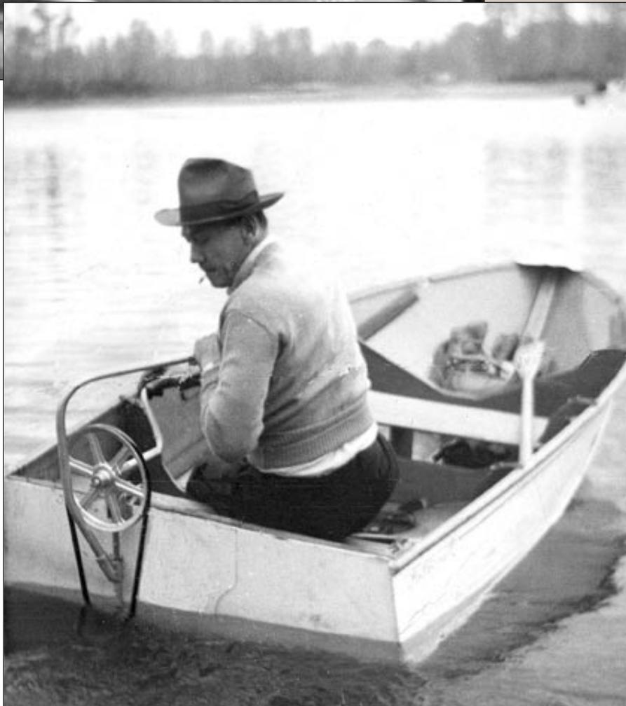
*Inventor Ben Randrup demonstrates the ill-fated Foldcraft boat with hand-operated propeller and handle for rudder in 1946.*
