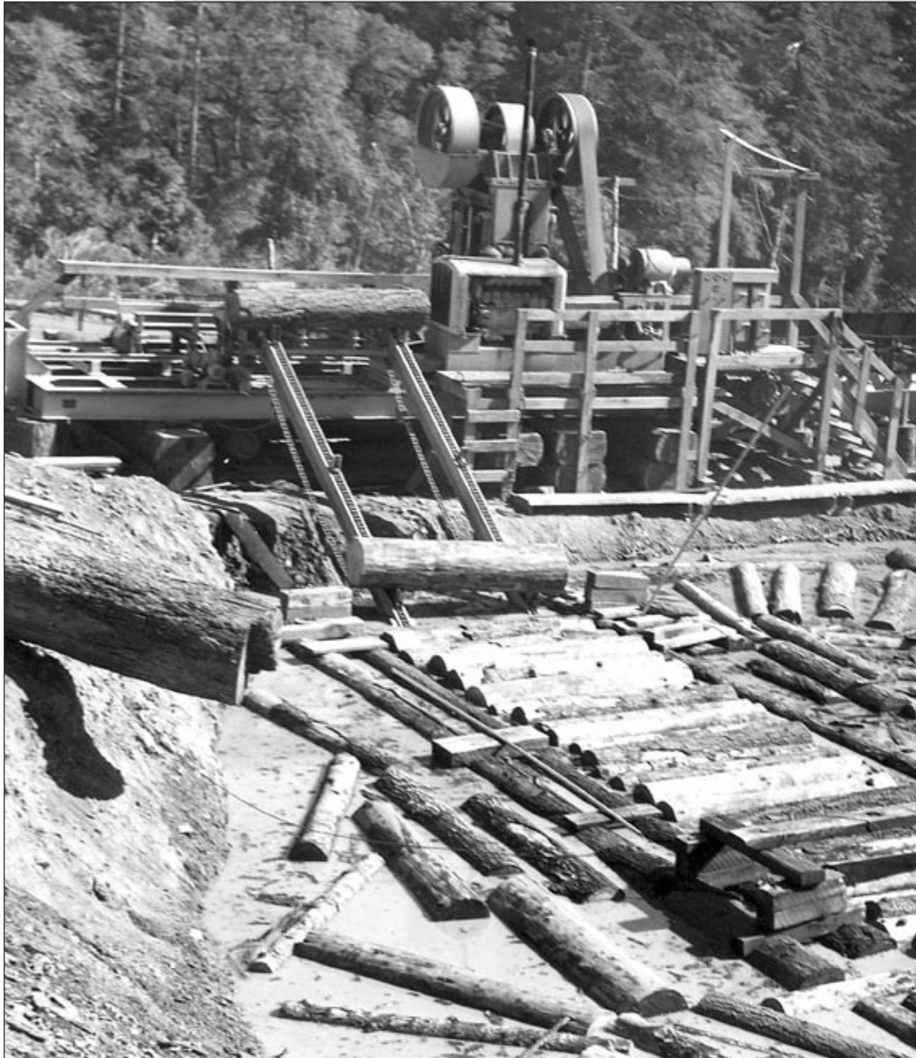
*During the late 1940s and early 1950s, Gunderson built logging machinery such as this 8' stud gang mill for McL Logging Company, Petrolia, California.*
