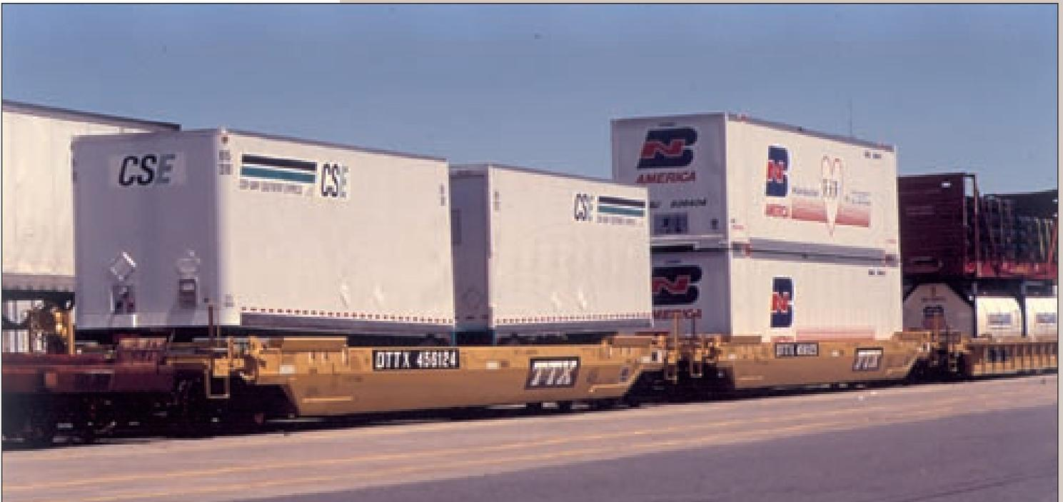
*Gunderson introduced Husky-Stack® in 1991, the first production version of a stand-alone double-stack car which has a higher load capacity. This version of the car, the All-Purpose Husky-Stack, can carry either trailers or double-stacked containers in the well.*
