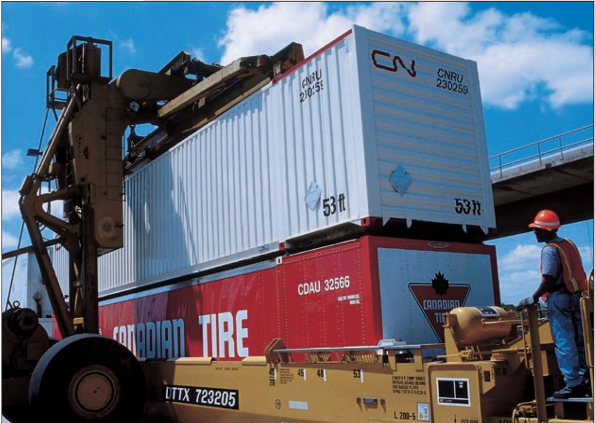
Gundersen's latest Maxi-Stack IV features 53-foot wells. Here, a TTX car is being loaded with 53-foot containers at Atlanta Georgia in preparation for the 1999 International Intermodal EXPO.
