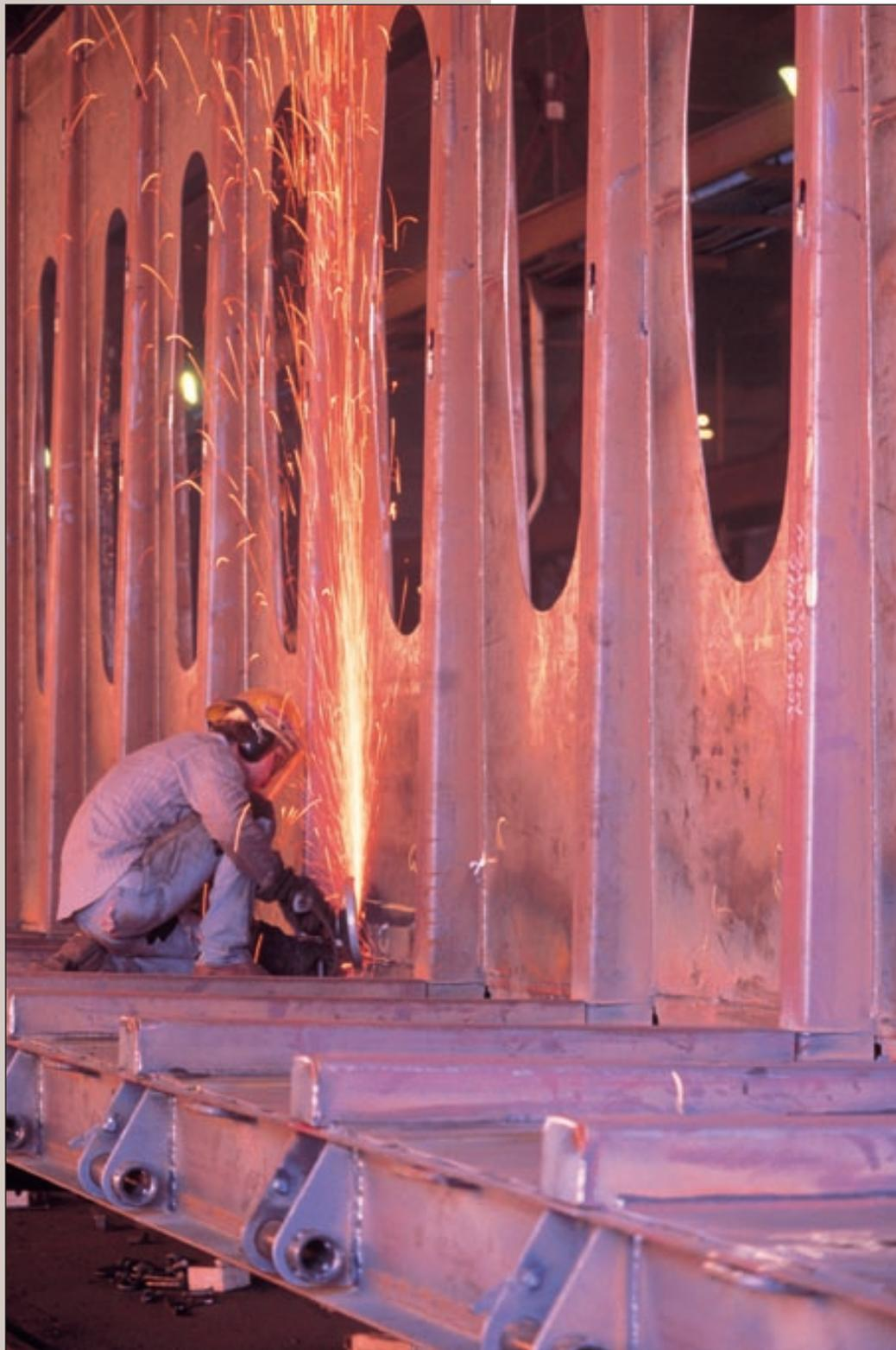
*A Gunderson worker grinds a weld smooth on a 73-foot center partition car during a production run in the late 1980's.*
